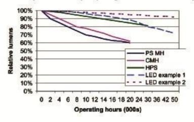
Figure 4. Typical lumen maintenance curves for HID sources, and estimated curves for LED.
