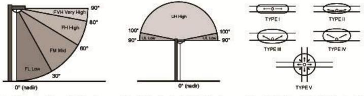
Figure 5. Section view for furward (F) solid angle. Light emmitted at high and very high angles can cause discomfort and disability glace for roadway users. Used with permission of IESNA.
